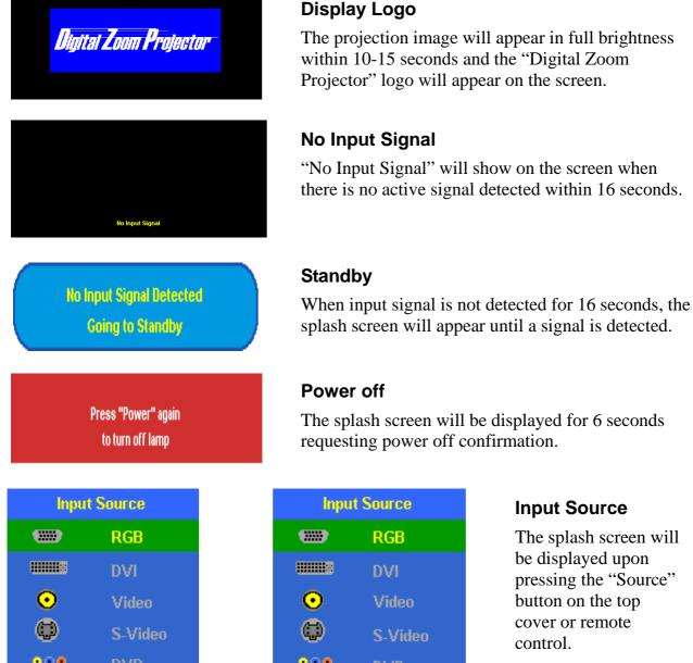
Press "▼▲" or "Source" to select the desired input source.
